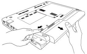
(Sample Illustration) Removing the battery
